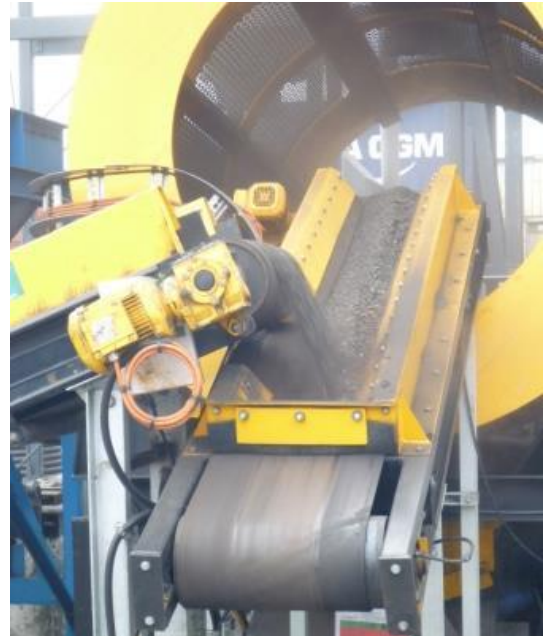
Feeding mill scale into the trommel.
