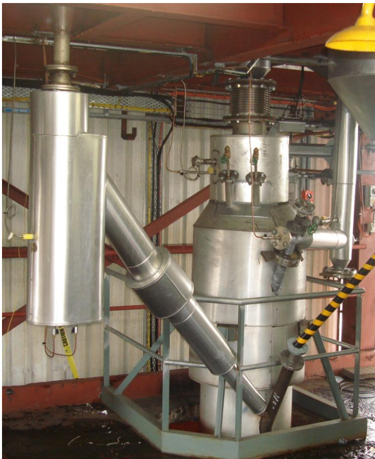
Ilmenite and Coal Feed and Cyclone Solids Return to the Reduction Roaster
