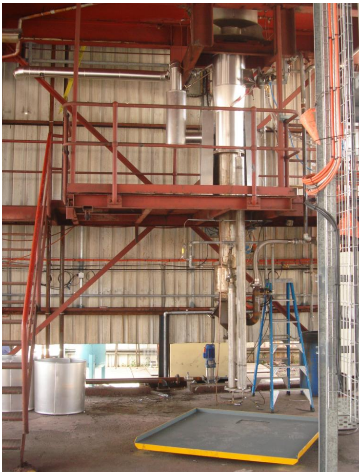
Roasted Ilmenite Cooler, Loop Seal Discharge and Roasted Product Weigh Scale
