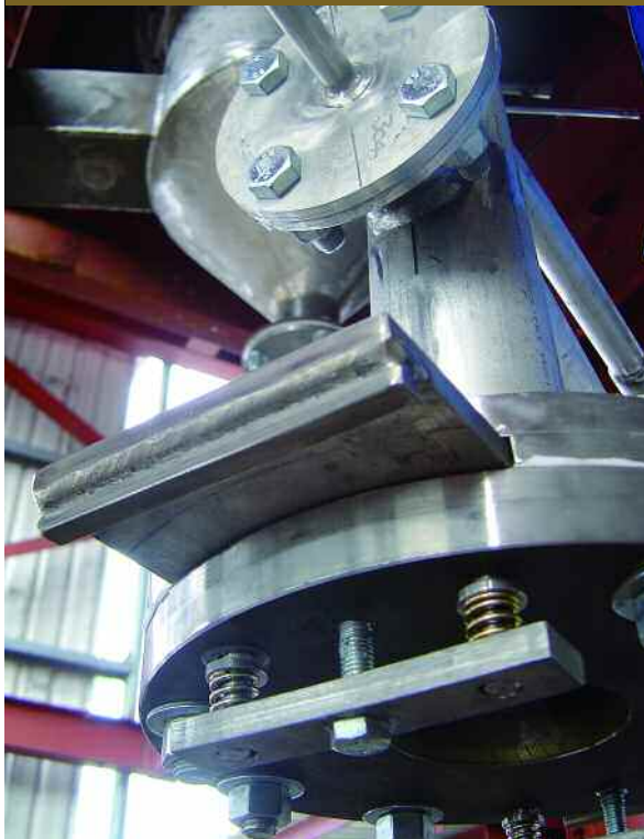
High temperature solids isolation valve
